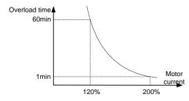
Fig 6.12-1 Motor overload curve
