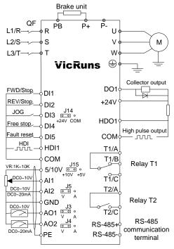
Fig 3.5-2 Standard Wiring Diagram for three-phase and lower than 15kW Inverter Precautions are as follows:
