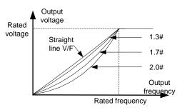
Fig 6.5-1 Schematic Diagram for Parabolic type
