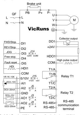
Fig 3.5-1 Standard Wiring Diagram for single phase 220V Inverter
