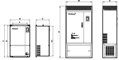
Fig2.6-3 Schematic Diagram for Physical Dimensions and Mounting Dimensions (up 132 kW)
