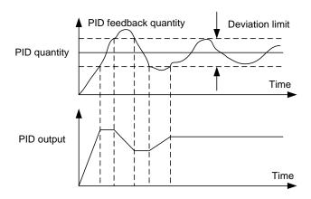
Fig. 6.8-3 PID deviation limit diagram
