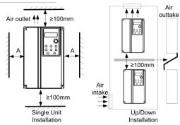
Fig.3-2-1 Inverter Installation Diagram
