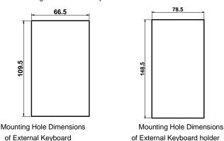
Fig.2.7-2 External keyboard and holder mounting dimension
