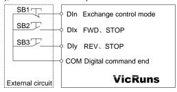
Fig 6.6-5 Alternate control mode
