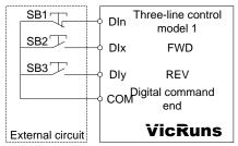
Fig 6.6-3 Three-line control mode 1
