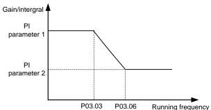
Fig 6.4-1Schematic Diagram for speed loop parameter switchover
