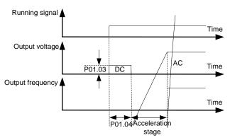
Fig 6.2-2 Schematic diagram for the braking current before starting
