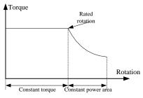
Fig 6.4-3 Weak magnetic function diagram
