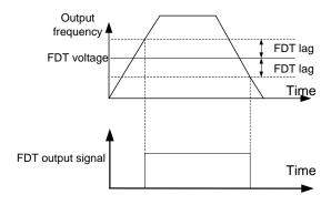
Fig 6.9-2 FDT signal diagram
