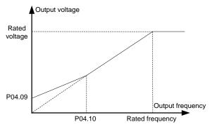
Fig 6.5-3 Schematic Diagram for torque boost
