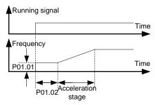
Fig 6.2-1 Schematic diagram for startup frequency
