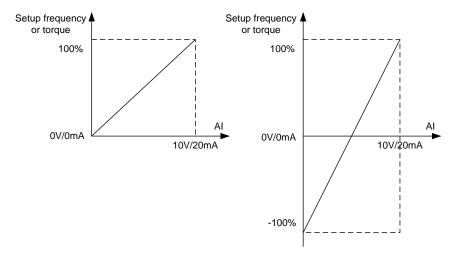
Fig.6.6-7 Corresponding Relationship between Analog Reference and Setting
