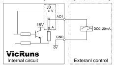
Fig 3.7-12 Schematic Diagram of Terminal of analog output of current signal 3.7.5.6 Output Terminals of Relay
