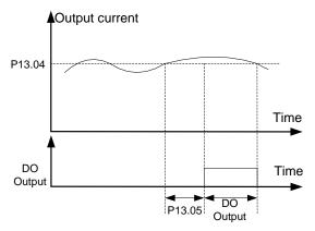
FIG 6.12-2 Detection of overload pre-alarm
