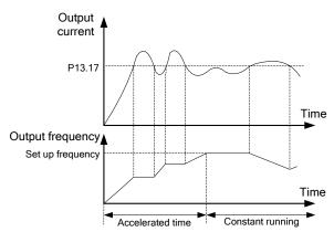
Fig 6.12-6 Diagram for over-current stall protection
