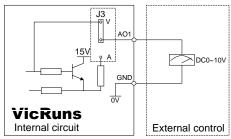
Fig 3.7-11 Schematic Diagram of analog output of voltage signal
