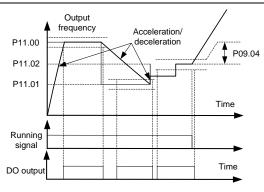
Fig 6.9-1 Diagram of Setting frequency arriving detecting amplitude
