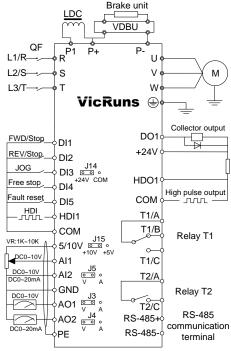
Fig 3.5-3 Standard Wiring Diagram for three-phase and higher than 18.5kW Inverter Precautions are as follows:
