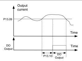
FIG 6.12-4 Diagram of output current over limit detecting
