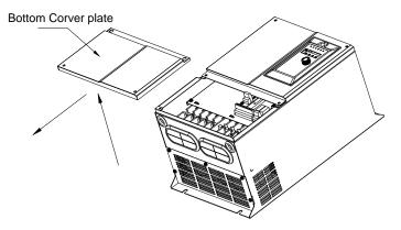
Fig 3.3-3 Removing and Installing the Cover Plate of Sheet-Metal Enclosure
