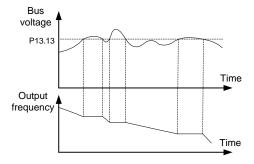
Fig 6.12-5 Diagram of over voltage under speed
