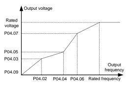
Fig 6.5-2 Schematic Diagram for MS V/F Curve
