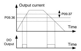
Fig 6.9-7 Random arrival current detecting diagram
