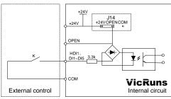
Fig 3.7-2 Schematic Diagram for Connection of Terminal of digital Input
