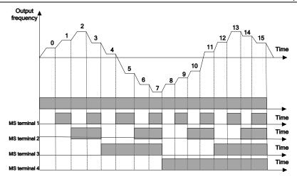
Fig 6.12-1 Multistage speed operation schematic diagram
