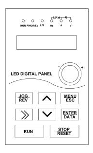
Fig.4.1-1 Operation panel schematic
