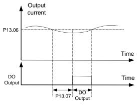
FIG 6.12-3 Offload pre-alarm detection
