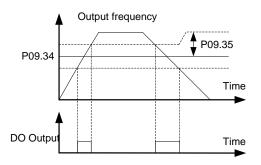
Fig 6.9-6 random arrival frequency detecting diagram
