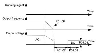
Fig6.2-3 Schematic diagram for DC braking time at stop
