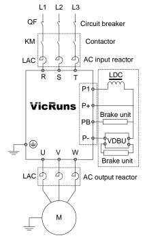
Fig 3.4-1 Inverter and external units electrical parts diagram
