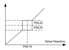
Fig6.9-4 Schematic diagram for Jump frequency
