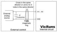
Fig.3.7-6 Schematic Diagram of analog input terminal cable jacket ferrite magnetic ring 3.7.5.3 Digital Output Terminal Using Internal Power Supply
