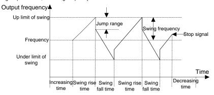
Fig 6.9-3 Schematic diagram for swing frequency work principle
